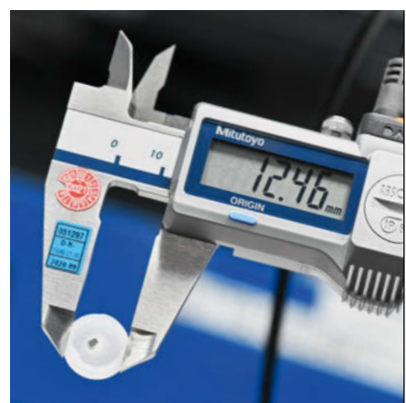
The sophisticated nanosensor with a magnet in the centre and a diameter of around 12.5 millimetres (images above) is produced on a turnkey system that is manually loaded with magnetic magazines (left image).
