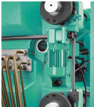
Interesting details of scale: drive unit for mould height adjustment.
