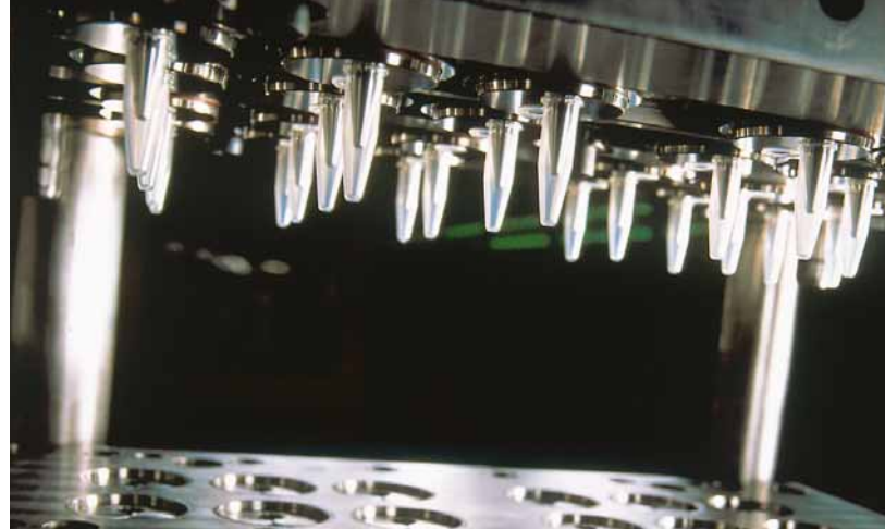
High-quality disposable products from plastic are manufactured in multiple cavity moulds.
