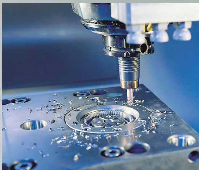
Electrode and mould processing in the company's own mould construction division. Photo: Bauser
