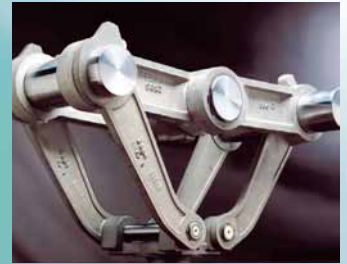
Robust, durable and economical: The well-proven ALLROUNDER toggle lever technology
