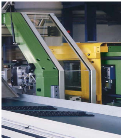
Automatic transportation of the encapsulated parts via a cooling conveyor belt
