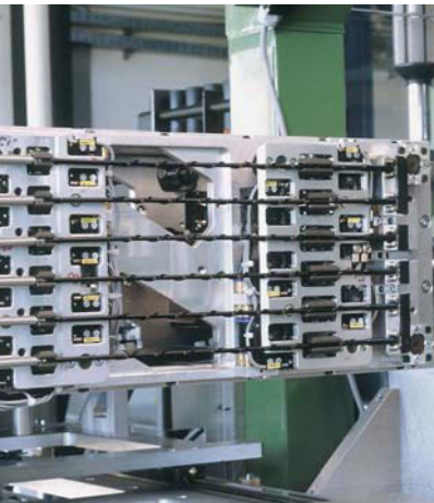
Six-way receivers for the antenna encapsulation
