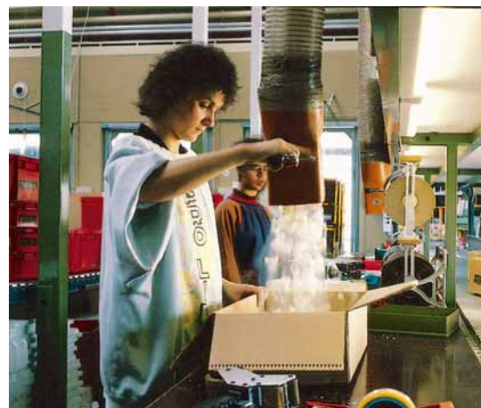
Recycled packaging materials are used to manufacture wadding to ensure safe delivery of spares
