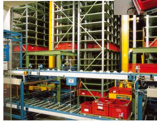
Completely computer-controlled Ordered parts are retrieved from storage without human intervention
