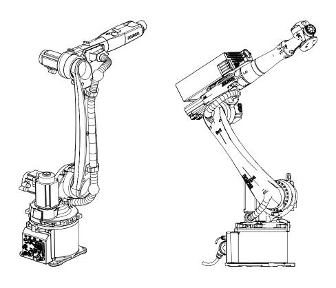
KUKA – POWERED BY ARBURG Handling weight: 6-120 kg
