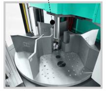
Tie-bar-free rotary tables of the V and T series: plenty of room for moulds and media connections.
