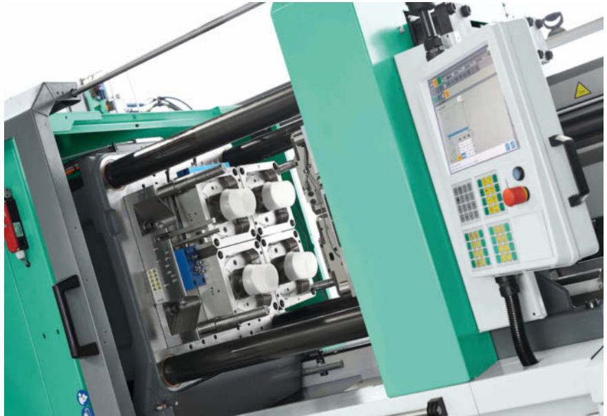
Fig. 1. Typical for high-speed applications with short injections times are thin-walled items such as round cups, here with a 4-cavity test mold © Arburg
